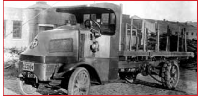
AC Model Can Haul Up To 7.5 Tons
